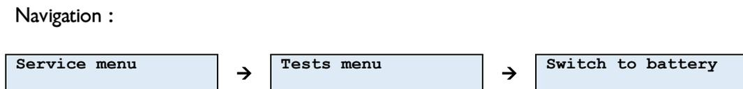
This test forces the U•V6 unit to switch to battery power, as if there were a mains power outage.
